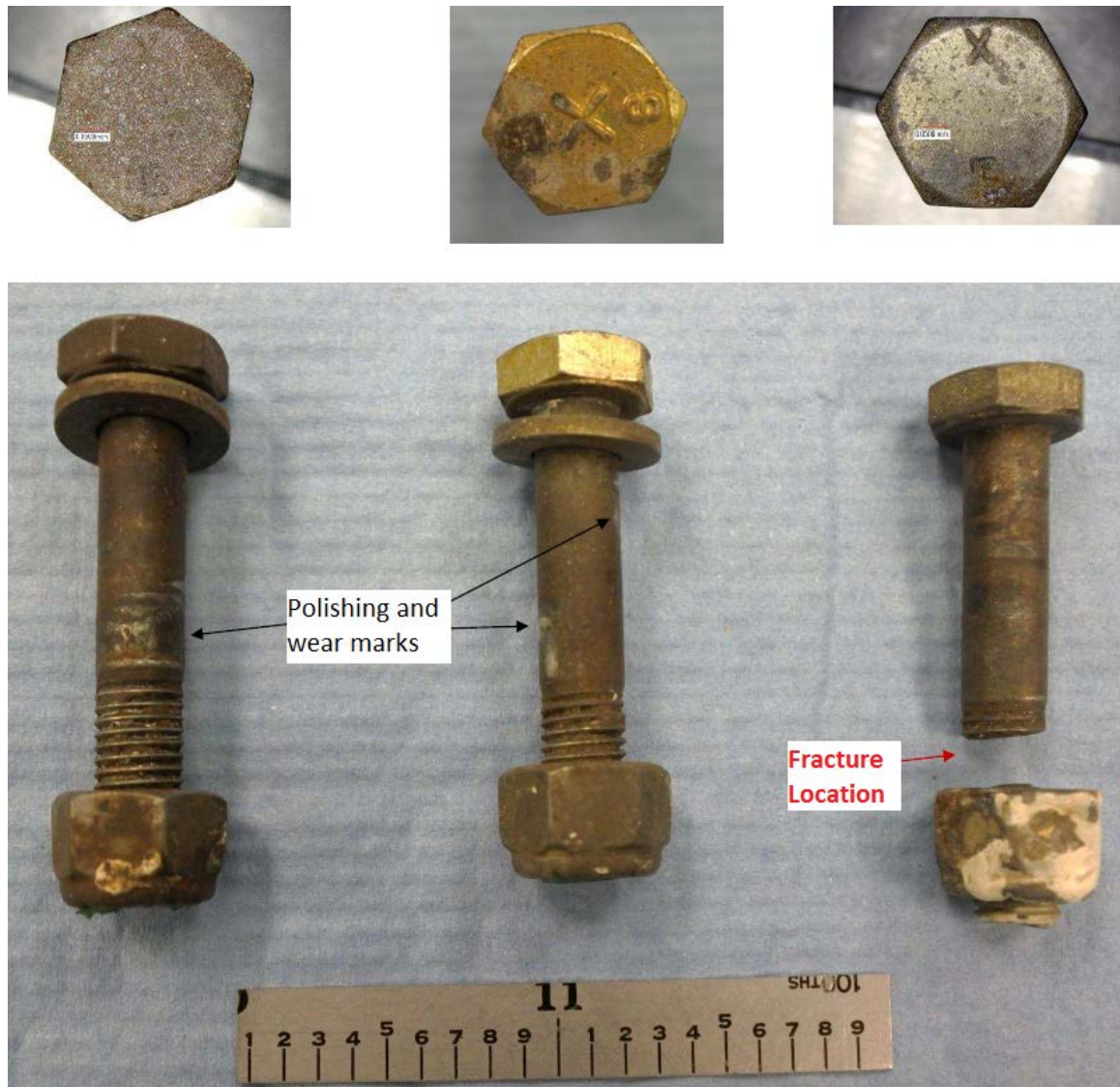
Figure 1 Horizontal Stabilizer Mount Bolts (P/N: AN4-12A). See Figure 6 (green arrows)
