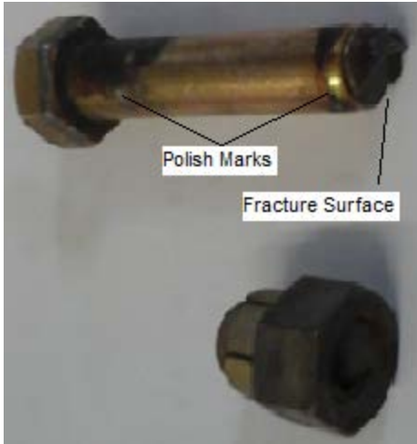
Figure 2 Polish Marks and Fracture Surface on Bolt, Found in April 2017
